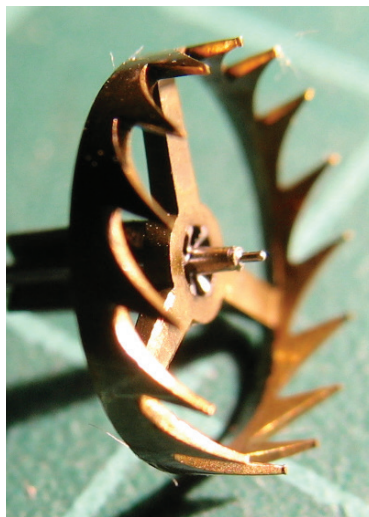
▲ Figure 21. LeRoy watch no. 687, detailed view of crown/escape wheel with 15 teeth, which engage with the two pallets on the verge staff. AUTHOR'S COLLECTION.
