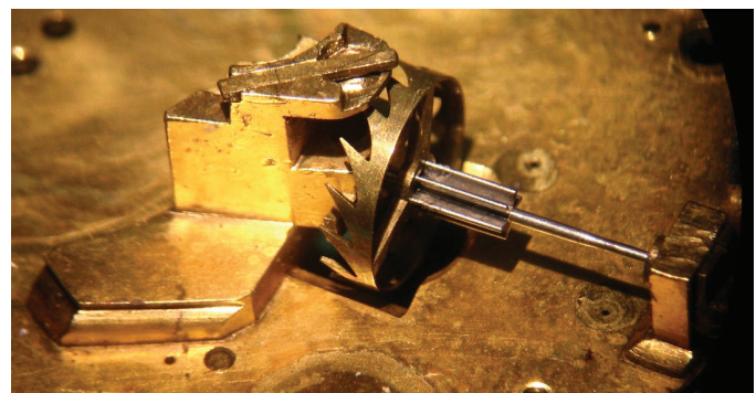
▲ Figure 15. LeRoy watch no. 687, detailed view of potence (left), counter-potence (right), and crown/escape wheel, showing quality of construction and finish. AUTHOR'S COLLECTION.
