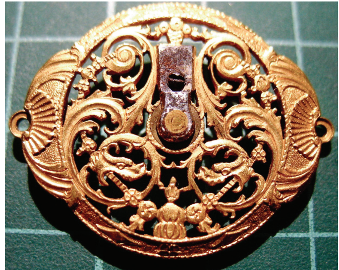
▲ Figure 13. A close-up view of the balance-cock (early Louis XV style) of the watch movement no. 687 by Pierre-François LeRoy, ca. 1730. As found, the steel cockerel needs cleaning. AUTHOR'S COLLECTION.
