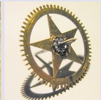
Figure 14. Caron watch no. 1244, detailed view of star-spoked center wheel. AUTHOR'S COLLECTION.
