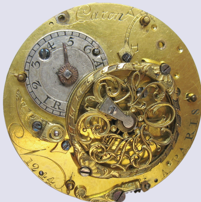
Figure 10. A view of the balance-cock side of the watch movement no. 1244 by André-Charles Caron, circa 1750. AUTHOR'S COLLECTION.
