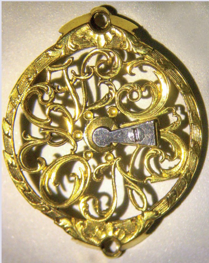
Figure 11. Caron watch no. 1244, detailed view of balance cock spelling Caron's name. AUTHOR'S COLLECTION.
