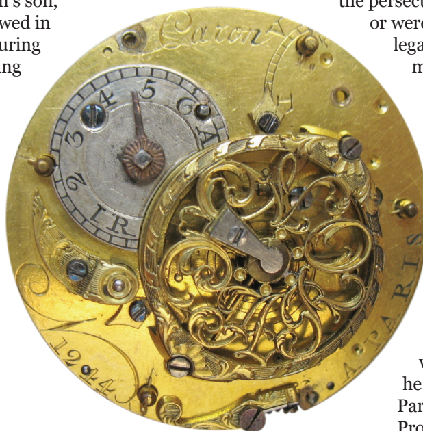
Figure 1. A view of the balance-cock side of the watch movement no. 1244 by André Charles Caron, circa 1750. Author’s collection.
